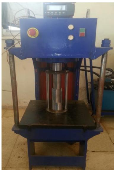
Figure 2 Hydraulic press and a punch-die set
