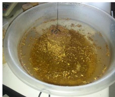
Figure 7 View of pepper crop briquette after water resistance test
