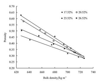
Figure 5 Porosity of acha at various moisture contents and bulk densities
