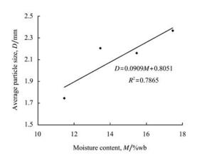
Figure 3 Plot of average particle size (D) against moisture content (M) for acha grains
