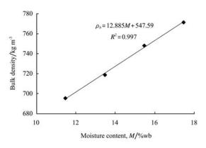
Figure 4 Plot of bulk density  $(\rho_b)$  against moisture content (M)
