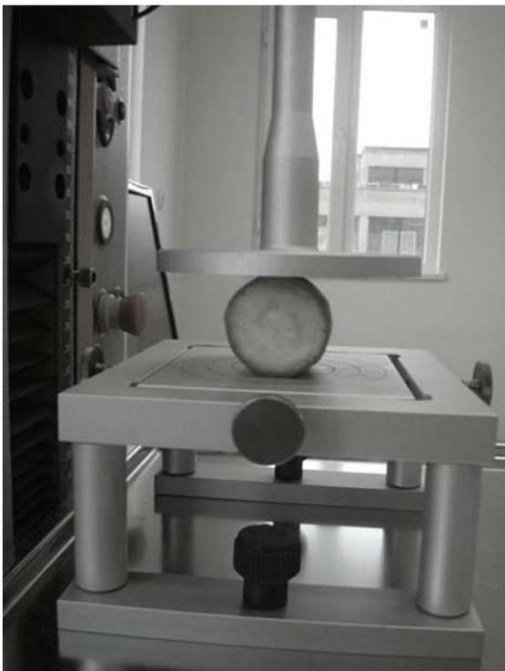
Figure 1 Zwick/roell universal testing machine equipped with a 500 N load cell
