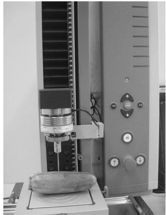
Figure 2 Specific device for measured penetration force
