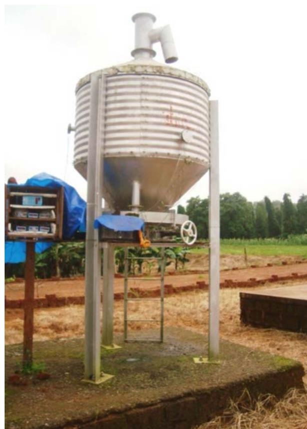
Figure 1 Galvanized iron corrugated structure for storage of wheat
