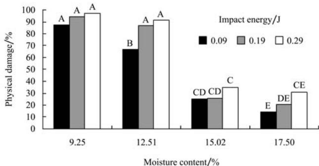
Figure 3 Effect of moisture content and impact energy interactions on percentage of physical damage to beans
