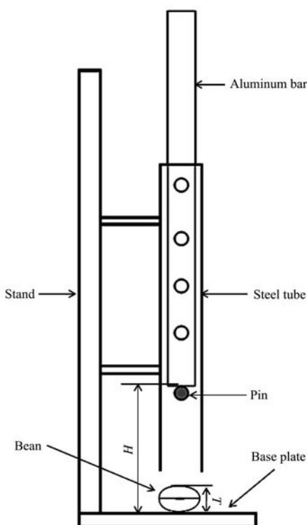
Figure 2 Schematic diagram of the impact test apparatus
