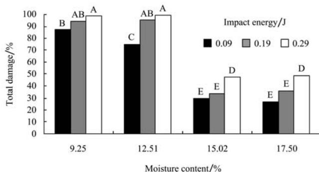
Figure 5 Interaction effects of moisture content and impact energy on the total damage to beans
