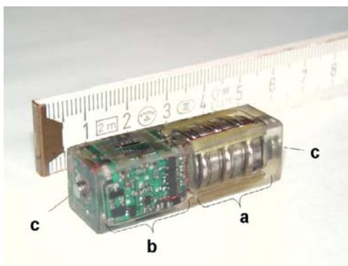
Figure 3.1. The acceleration measuring unit (AMU): a =battery, b= electronic circuitry with acceleration sensor, data processor, and data transmitter, and c = contact points for recharging.
