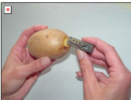
Figure 3.2. Implantation of the AMU into a potato tuber.
