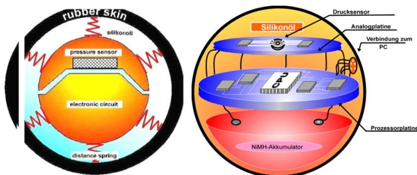
Figure 2.3 Internal electronic units of the PMS-60.
