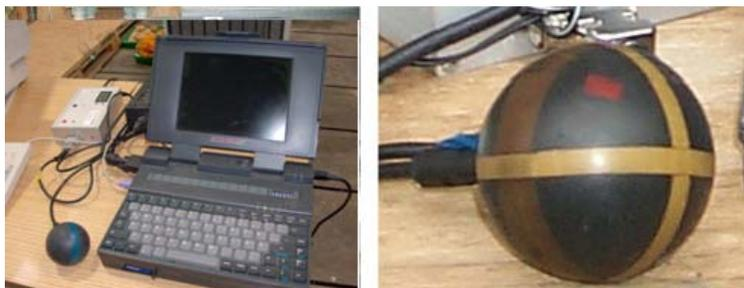
Figure 2.1 Pressure Measuring Sphere PMS-60 to measure fruit impact forces on-line.
