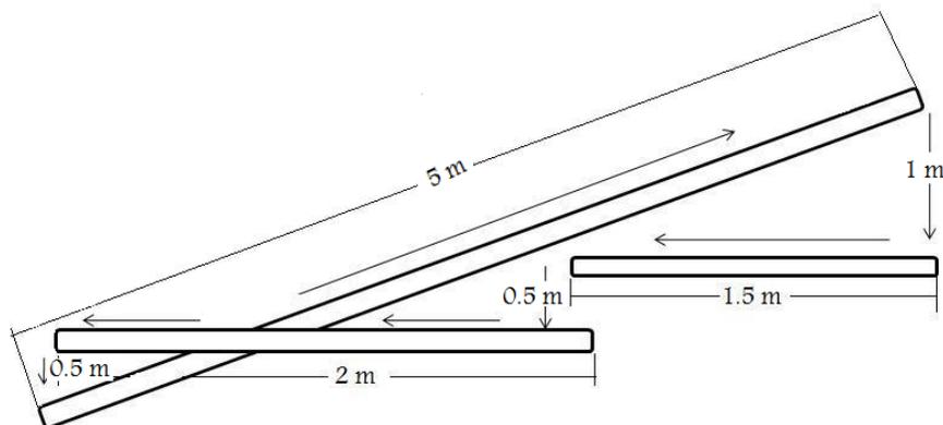
Figure 1. Schematic view of the processing line simulator test device with three conveyor belts running in circuit.
