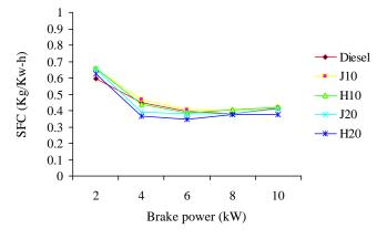
Figure 4 Variation of specific fuel consumption with load
