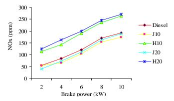
Figure 7 Variation of NO<sub>x</sub> emission with load
