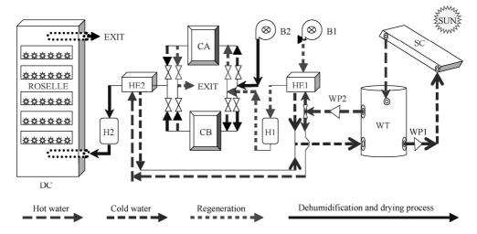
B = air blower; CA = column A; CB = column B; DC = drying chamber; H = heater; HE = heat exchanger; SC = solar collector; WP = water pump; WT = water tank
