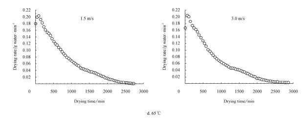
Figure 7 Drying rate (DR) at 35°C, 45°C, 55°C and 65°C
