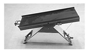
Figure 4. Apparatus for measuring static coefficient of friction.
