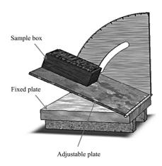
Figure 3 Apparatus for measuring the angle of repose
