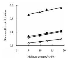
Figure 13. Effect of moisture content on static coefficient of friction: (•) galvanized iron sheet; (ο) mild steel, (Δ) plywood and (Δ) aluminum
