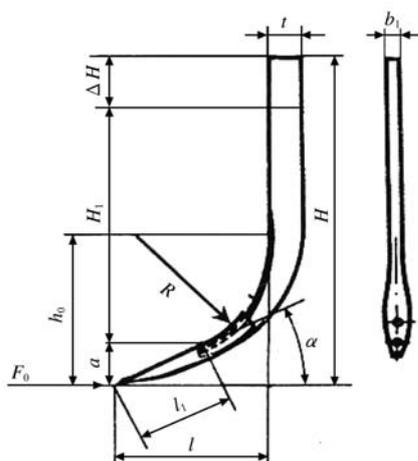
Figure 4 Dimension of tine of furrow opener
