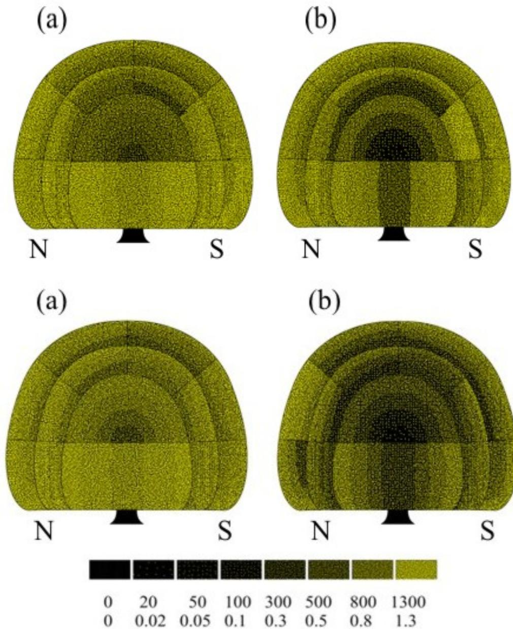
Figure 5. Comparison of droplet deposition on citrus leaves using a multi-fan spray tower with spray heads arranged in 3 horizontally converging pairs (upper diagrams) with a tower with heads in a simple vertical array (lower diagrams). (a) upper leaf surface; (b) lower leaf surface. Bar legend: upper scale – estimated droplet number  $\text{cm}^{-2}$ ; lower scale – estimated deposit volume ( $\mu\text{L cm}^{-2}$ ).
