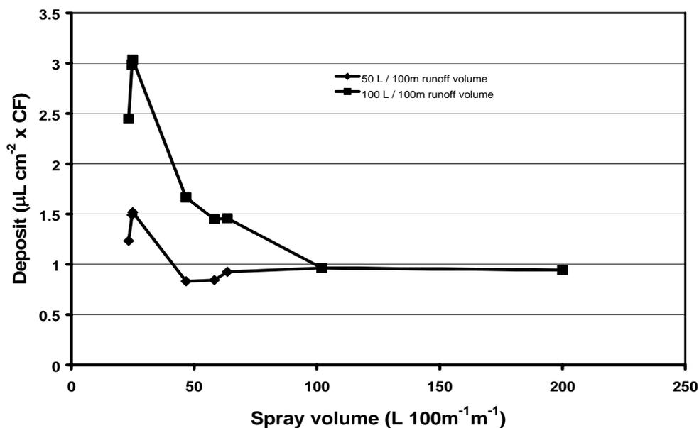
Figure 2. The effect of spray volume on spray deposition on citrus leaves with concentrate spraying. (a) Liquid volume, (b) Estimated relative mean deposit with concentrate spraying using a concentration factor based on a run off volume of  $50 \text{ L } 100 \text{ m}^{-1} \text{ m}^{-1}$  (diamond points) and  $100 \text{ L } 100 \text{ m}^{-1} \text{ m}^{-1}$  (square points). Concentration factor above run off volume = 1.
