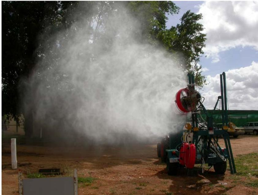
Figure 1. Multi-fan tower sprayers. (a) Commercial citrus tower sprayer with 4 heads per side. (b) Prototype Sprayer showing one of the horizontally converging pairs of spray heads. (c) Prototype sprayer with one pair of horizontally converging spray heads operating, showing the vertical fan pattern produced.
