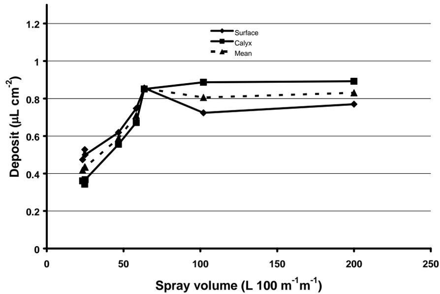
Figure 3. The effect of spray volume on the liquid volume deposited on citrus fruit.
