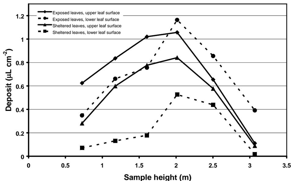
Figure 6. Liquid volumes deposited in the outer canopy of citrus trees sprayed with a single pair of horizontally converging spray heads.
