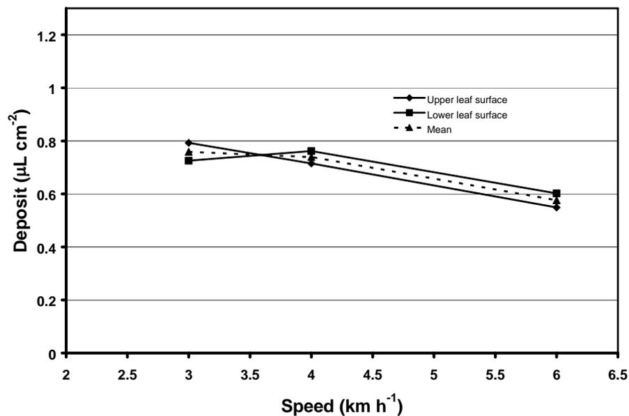
Figure 4. Effect of spraying speed on the liquid volume deposited on citrus leaves using a multi-fan tower sprayer to apply a spray volume of  $25 \text{ L } 100\text{m}^{-1}\text{m}^{-1}$ .
