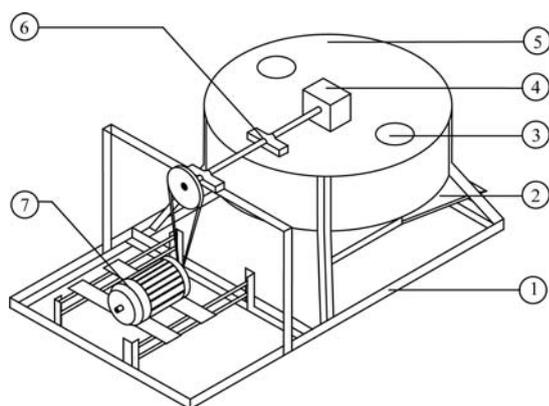
1. Device Frame 2. Collector 3. Feeding Chute 4. Gear Box
