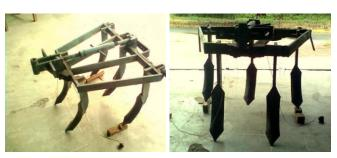
Figure 1 The 5-tyne cultivator prototype with isometric and front view
