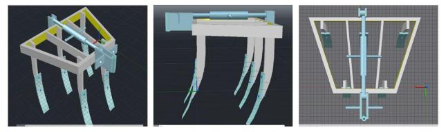
Figure 2 AutoCAD model of 5-tyne cultivator
