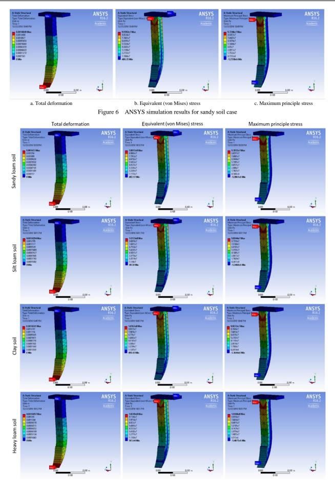
Figure 7 ANSYS simulation results of total deformation, equivalent (von Mises) stress, and maximum principle stress for sandy loam, silt loam, clay and heavy loam soil test cases. Each row represents results for each test case. Max and Min tags in each results showing maximum and minimum value of the output
