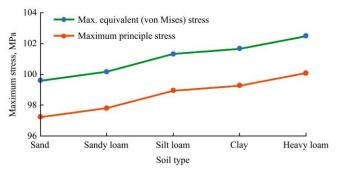
Figure 8 Maximum stress for different soil condition based on ANSYS simulation output
