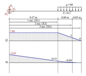
Figure 4 Shear force  $(Q_y)$  and bending moment  $(M_x)$  diagram of cultivator tyne considering, Cultivator tyne as a cantilever beam fixed at point A. Cultivator self-load, P<sub>1</sub>=0.1 kN and soil resistive force  $(q_1)$  as a distributed load of 60 kN m<sup>-1</sup> on type
